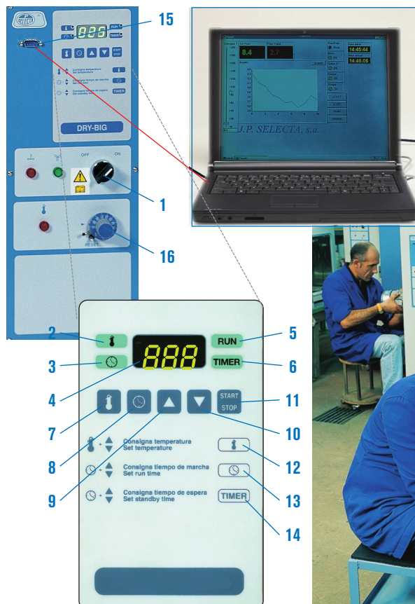
Oven's diagram seen from the front side.
