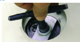
Orbital rotation adjustment
